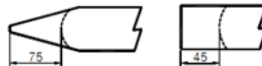
Flat type rod worn more than 45mm or moil type and wedge, universal type rods worn back more than 75mm of working end classed as reasonable life. Warranty claims rejected.
